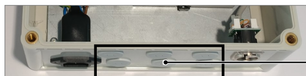
Fig 39. Remove Cable Cover Plugs
